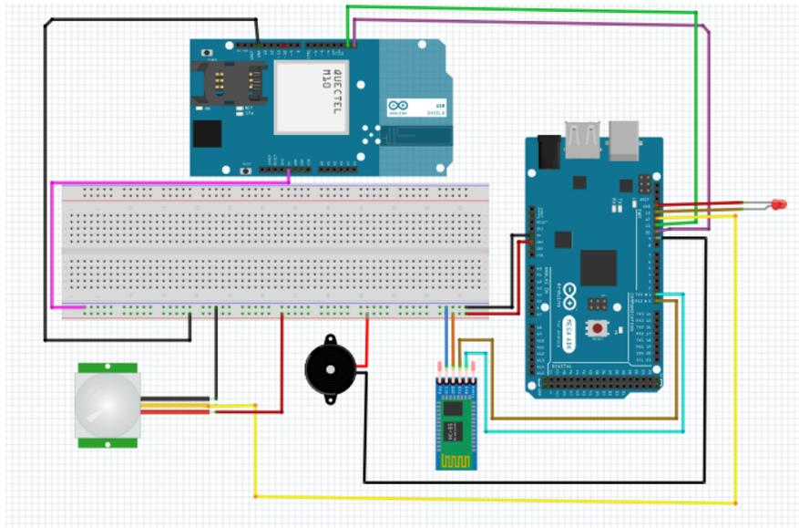
**Figure 3.** System design of the remote home security
